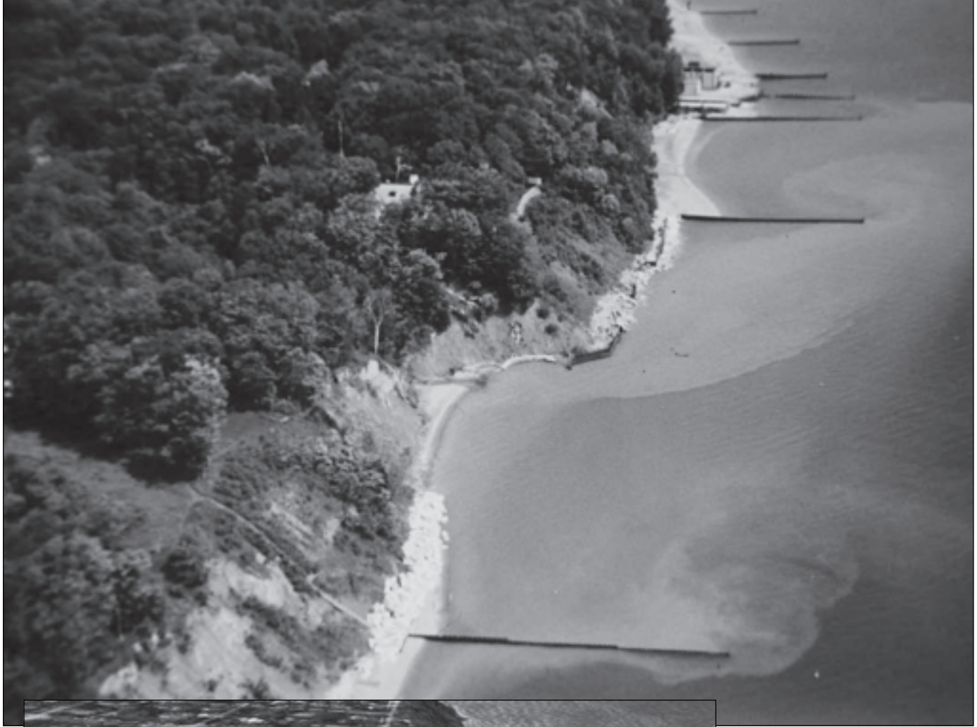
Figure 2. Lake Bluff Ravine Park Ravine. Mouth of ravine and lakeshore prior to (1990, above) and after ravine and beach restoration (2009 Google photo, left). Note sediment plume from eroding ravine and adjacent bluffs. The pocket beach and wetland protecting the ravine mouth lie at the downdrift end of a series of pocket beaches that have replaced the poorly functioning groin field.
