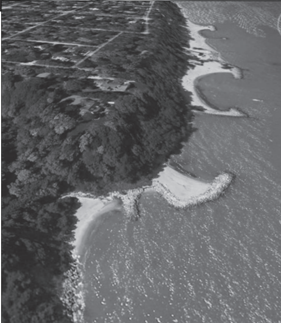
Figure 2. Lake Bluff Ravine Park Ravine. Mouth of ravine and lakeshore prior to (1990, above) and after ravine and beach restoration (2009 Google photo, left). Note sediment plume from eroding ravine and adjacent bluffs. The pocket beach and wetland protecting the ravine mouth lie at the downdrift end of a series of pocket beaches that have replaced the poorly functioning groin field.
